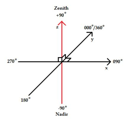
Bearing: denotes a direction, ranging in angles 000° through to 359° on the xy-plane
